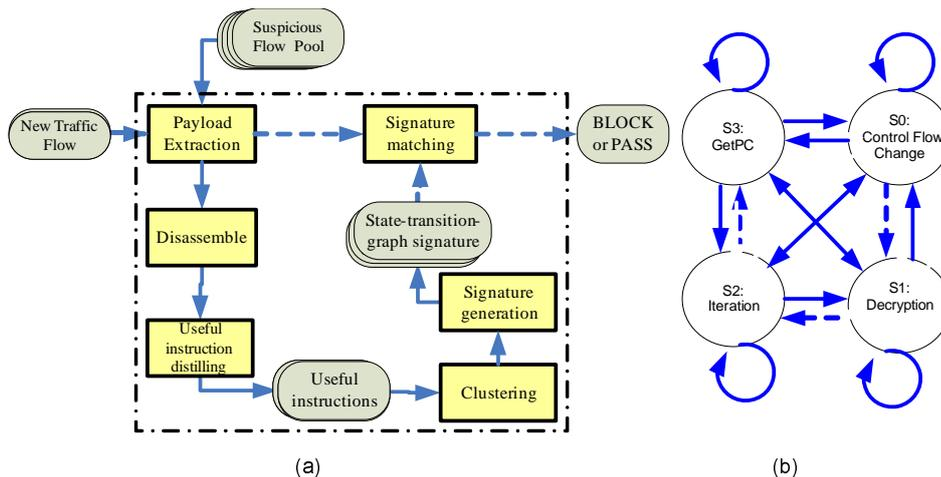
Fig. 2. (a) System architecture. (b) State-transition-graph (STG) model
