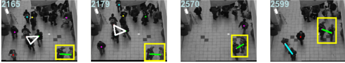
Figure 4. Sample group detection results in the SU1 sequence. Links between people denote hypothesized small groups. Notice that the group marked with the rectangle has been consistently identified throughout a change of status from stationary to moving.
