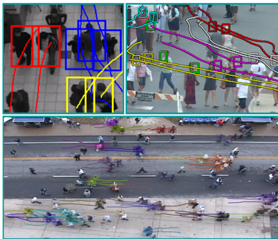
Figure 1. Small groups are prevalent in pedestrian scenes. Our algorithm detects groups of people traveling together via hierarchical clustering on trajectories automatically extracted from video of crowds under various conditions.
