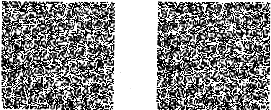
Fig. 1. Basic random stereo pair. When the two fields are viewed stereoscopically, the center square appears in front of the background. [See (7) for a description of an aid useful in stereoscopic viewing.]
