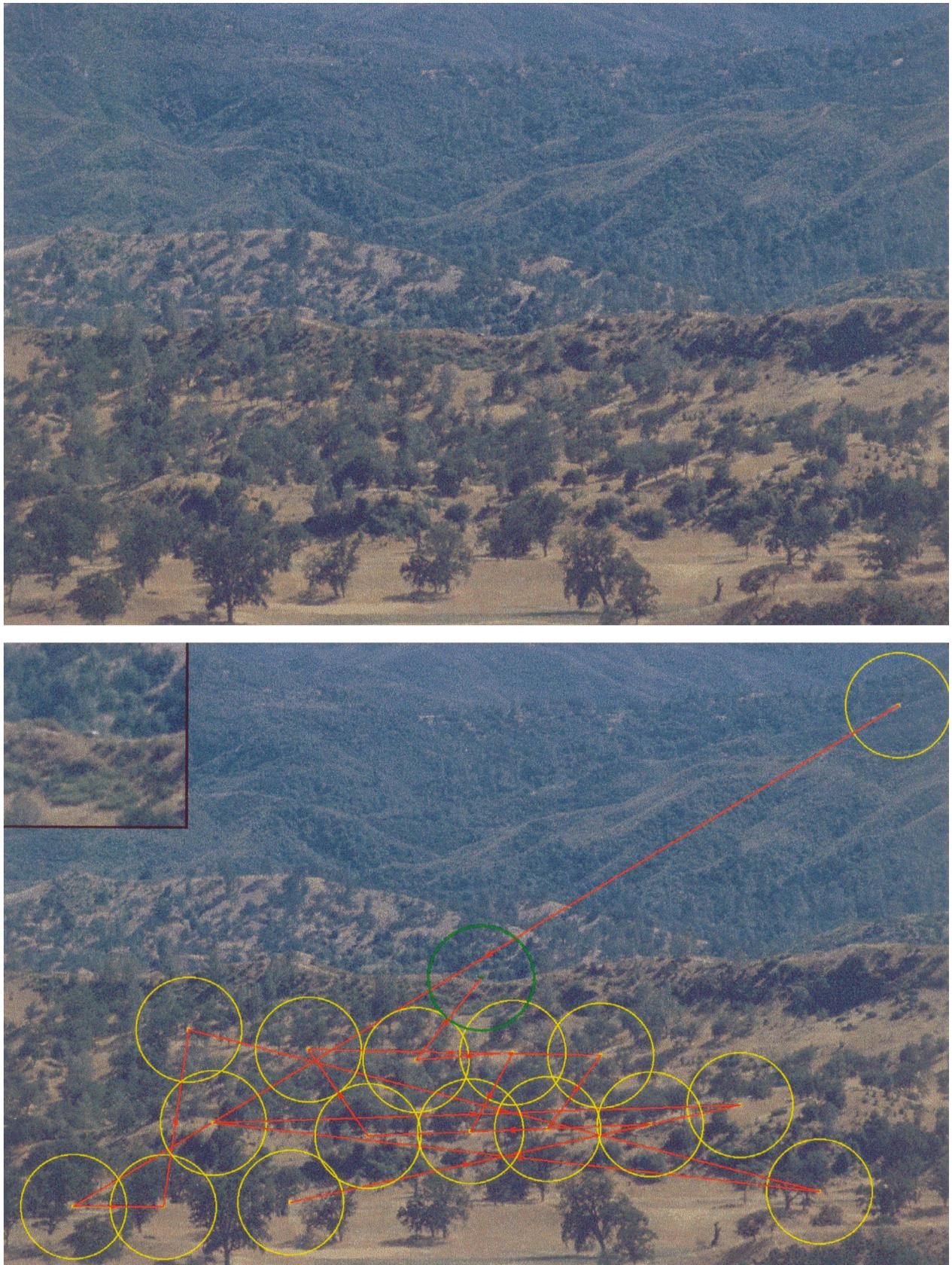
Fig. 7. A more difficult example from the image database studied. (a) A rendition of the color image. Humans found the location of the vehicle in 7.5 s on average. (b) The target is not the most salient object, and the model searches the scene in order of decreasing saliency. The algorithm came to rest on the location of the target on the 17th shift, after 6.1 s (using same time scaling as in the previous figure).
