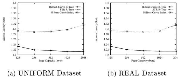
Figure 7: Access Latency of Different Indexing Structures for KNN Queries
