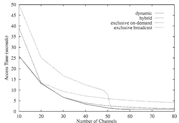
Figure 12. Access time vs. number of channels.
