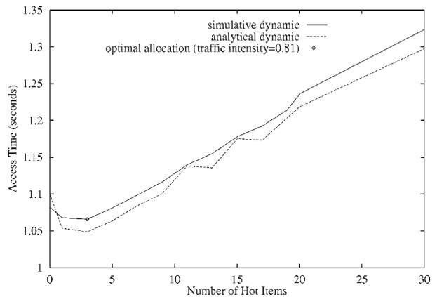
Figure 9. Optimal access time vs. number of hot items for a light-loaded system.
