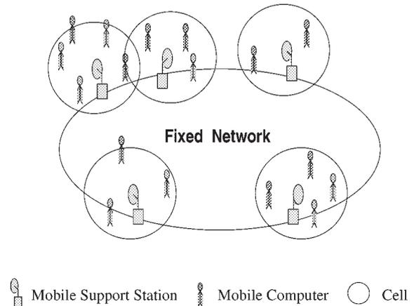
Figure 1. Mobile computing system.
