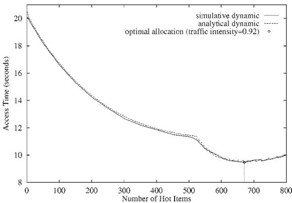
Figure 6. Optimal access time vs. number of hot items for a heavy-loaded system.
