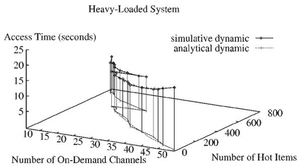
Figure 5. Optimal access time for a heavy-loaded system.
