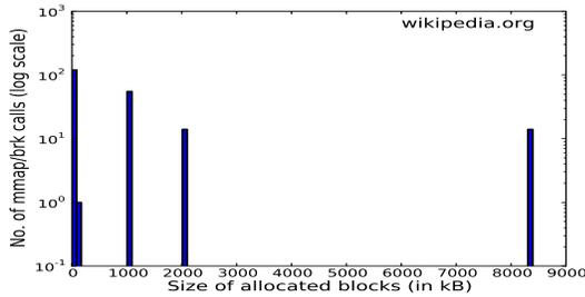
Figure 4. Firefox: Distribution of mmap/brk allocation sizes.
