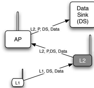
Fig. 2. A message is sent from an L1, translated by a NAT-like process in an L2 and forwarded from port  $P$  via an AP to its intended destination. Commands or requests from the data sink follow the reverse path, except that the traversal of the wired network may be different due to Mobile IP.
