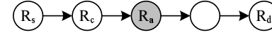
Figure 1: Injection attacks in a route, in which R_s is the source and R_d is the destination. An attacker R_a stays in the route and injects junk packets with the spoofed address of R_s . Because the route is used to forward packets from R_s to R_d , junk packets will be forwarded. The destination can trace the packet back along the route if it detects junk packets. Unfortunately, the trace goes back to the source R_s instead of the attacker R_a in the middle.
