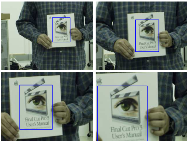
Figure 6: Similarity tracking with the multi kernel SSD approach. The first frame shows the selected template region. The subsequent frames show the tracked region with a blue rectangle
