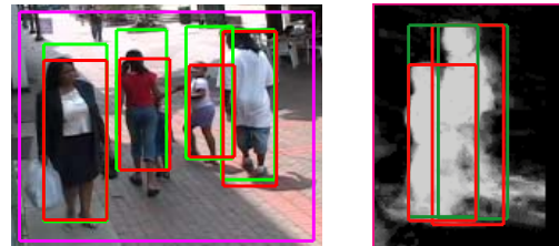
Figure 5: Shape Estimation. In a set of experiments one degree of freedom was added to the shape space so that children as well as adults can be segmented correctly. The initial shape of the clique is shown in green and final estimated size in red. Note that the algorithm accurately segments people of different heights.
