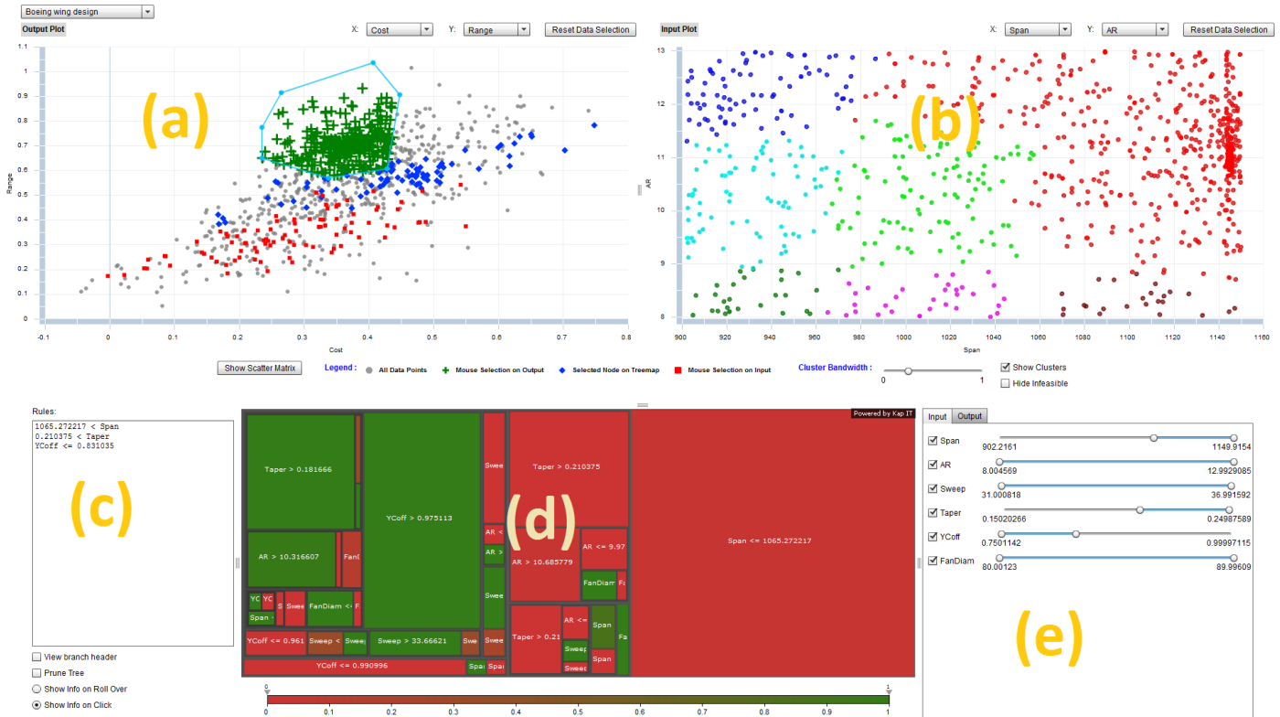
Figure 2. SCREENSHOT OF LIVE SYSTEM: (a) SCATTER PLOT OF PERFORMANCE OUTPUT VARIABLES; (b) SCATTER PLOT OF DESIGN INPUT VARIABLES (SHOWING CLUSTERING RESULTS); (c) TEXT REPRESENTATION OF DECISION RULES; (d) TREEMAP VISUALIZATION OF DECISION TREE; (e) ADJUSTABLE SLIDERS OF RANGES OF INPUT AND OUTPUT VARIABLES.
