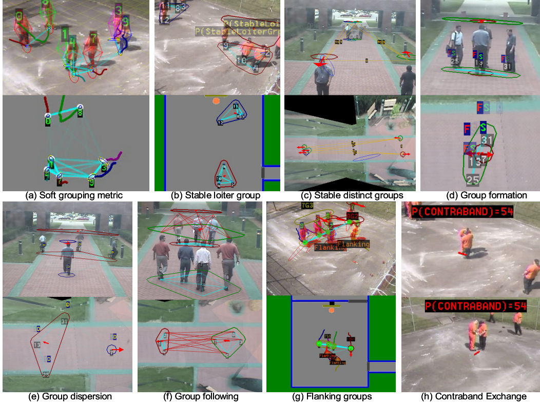
Figure 3. Snapshots of several group-level activities captured by our system, where in each case the top depicts one (out of many) camera views and the bottom depicts a top-down 2D planar view, except (h). (a) Cyan lines depict our probabilistic path-based grouping connectivity p_c^\pi as a complete graph of all tracks; lower transparency indicates higher probability. (b) Detected stable loitering groups, where the transparency indicates probability p_g^{sl} . (c) Three detected pairs of stable distinct groups, where each yellow edge depicts p_g^{s,d} . Observe that only people of different groups trigger strong signals. We denote ‘F’ in red for formation, ‘S’ in green for stable, and their transparency indicates probabilities p_g^f and p_g^s . (d) Detected group formation in the same sequence after (c), where the 4 people gather together such that their overall group size is increasing. We denote ‘F’ in red for formation, ‘S’ in green for stable, and their transparency indicates probabilities p_g^f and p_g^s . (e) Detected group dispersion in the same sequence after (d), where the 4 individuals disperse (‘D’ in yellow for p_g^d ). (f) Detected group following p_g^{flw} in red edges connecting two major groups, where one is following another. (g) Detected flanking maneuver, where 4 enacted inmates are surrounding 2 victims for an attack. Red circle indicates high probability of being flanked, while green circle indicates low probability. Observe that the grouping connectivity between members in the aggressive group is very strong. (h) Detected contraband exchange with a certain probability.
