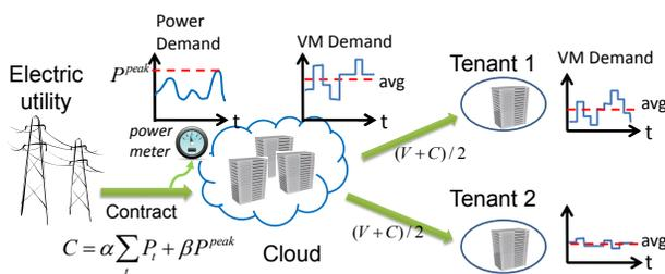
Figure 1: An example illustrating unfairness in how tenants with different demand variances are charged under a peak-based electricity pricing scheme. ( $V$ : VM cost charged by the cloud.)
