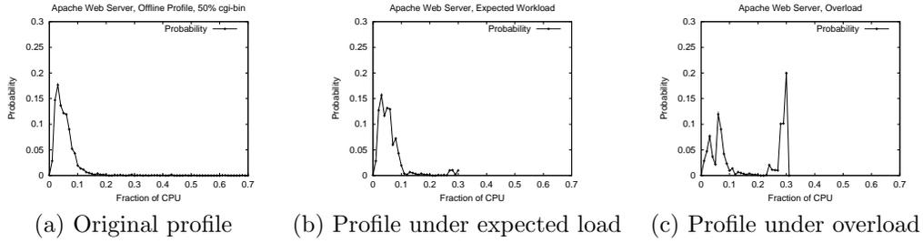
Fig. 8. Demonstration of how an application overload may be detected by comparing the latest resource usage profile with the original offline profile.
