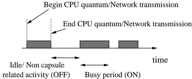
Fig. 1. An example of an On-Off trace.
