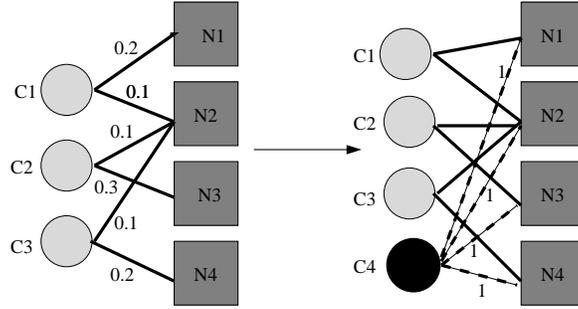
Fig. 7. Reducing Minimum-Weight Maximum Matching to Minimum-Weight Perfect Matching.
