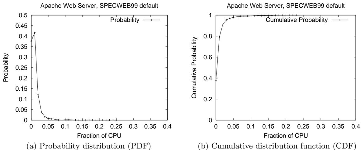
Fig. 3. Profile of the Apache Web server using the default SPECWeb99 configuration.
